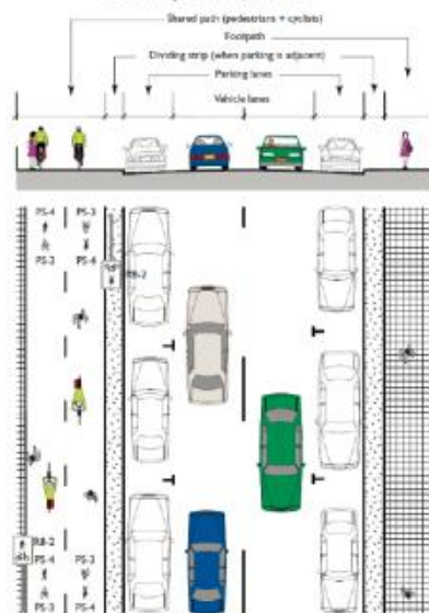
Figure 5.4: Potential facility and cross-section - Gauthorpe Street, Rhodes
